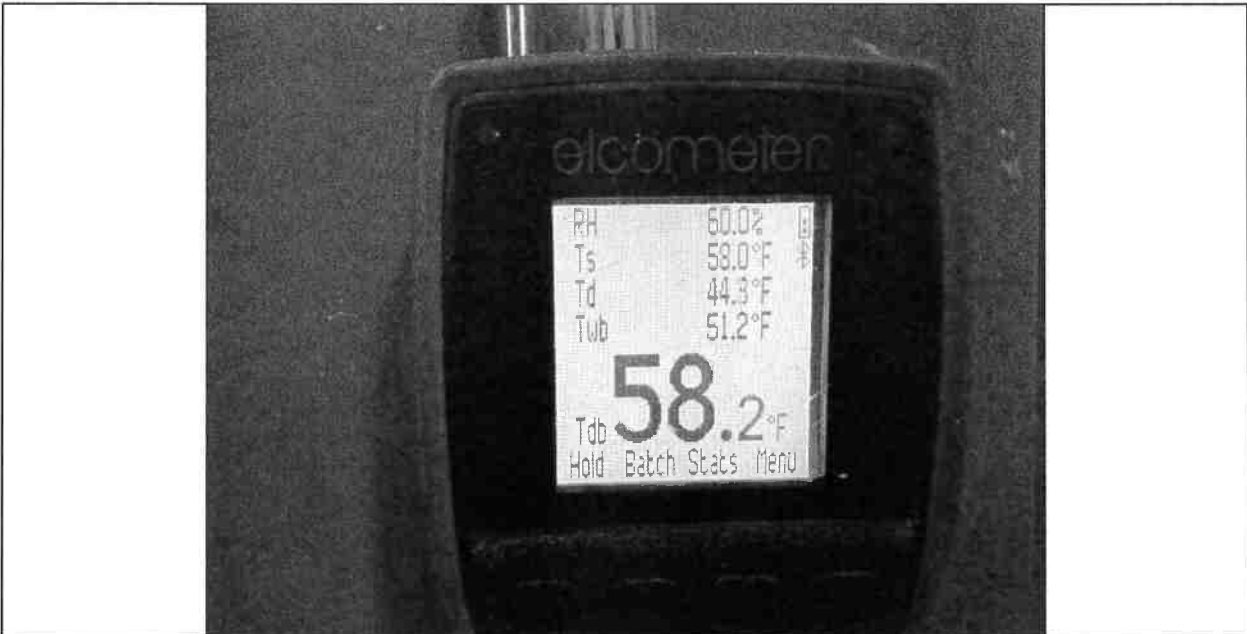
Interior Ambient temperatures prior to internal primer coating
