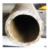
trict will be testing a total of six samples in different soil types within Centerville to evaluate the AC pipe's current condition as well as better forecast its remaining useful service life. This information will be helpful in planning for future pipeline rehabilitations and replacements.
