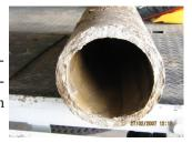
PACE Engineering, Inc. recommended that the District have the AC Pipe tested to determine its condition and estimate the remaining useful life of the pipe. The Board of Directors unanimously approved a proposal from Exponent for testing and analysis services. Total project cost: \$67,400.00.
